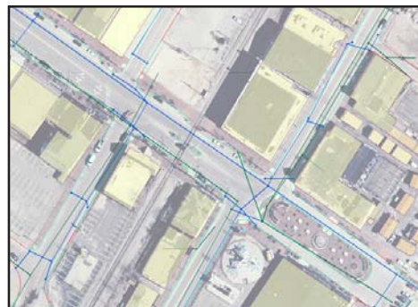
Infrastructure assets including manholes, catchbasins, and storm and sewer connectivity projected on the basemap.
